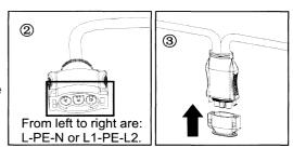
Step 7. Connect APsystems Microinverters to the PV Modules
