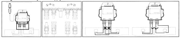
Step 8. Connect APsystems Microinverters to Grid
